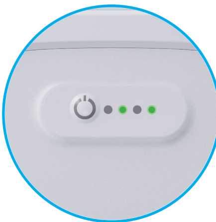
The 1st and 3rd LEDs are flashing
